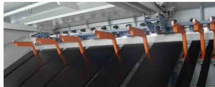
**Lever type pneumatic sheet support system (optional)**
