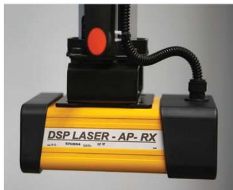
■ DSP MCS AP finger protection system making time saving easy (O)
