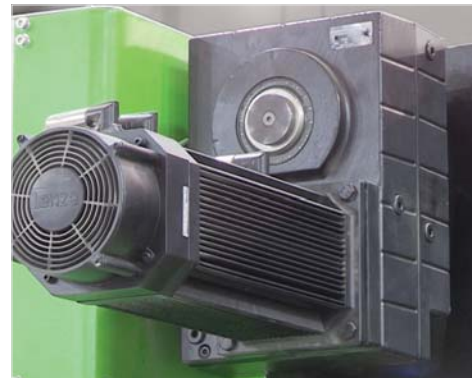
■ Top beam is moved with high efficient synchronous ac servo motors (S)
