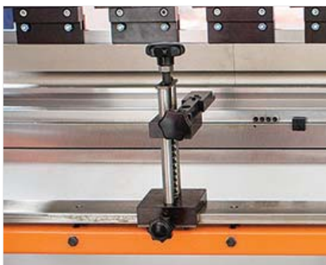
■ Specially designed folding backgauge fingers (S)
