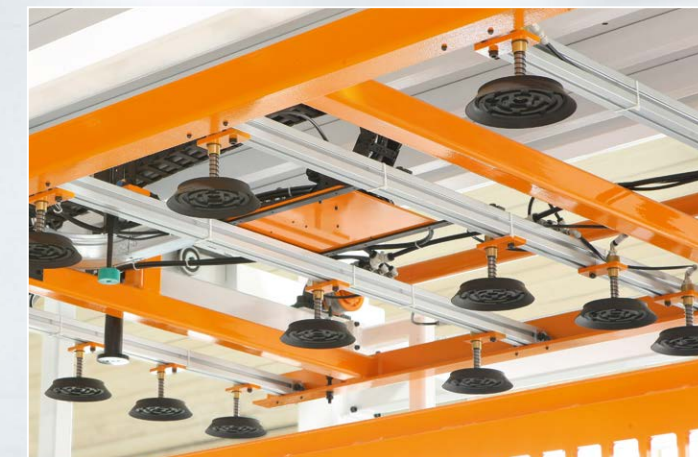
Suction cup device for lifting raw metal sheet: Is an arm with the grip placed over the loading pallet. The duty of this arm is to lift the raw metal sheet to permit the entrance of the comb device under the metal sheet lifter and deposit it on this comb device.
