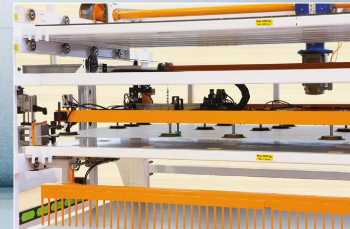
Stock Area: Automatic system handle the sheet and place it in the proper stock area.
